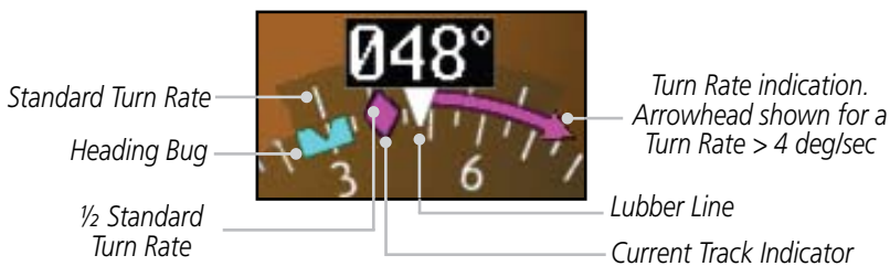
Figure 2-27 Turn Rate Indicator and Trend Vector
